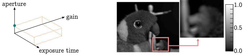
Figure 2.5 – Capturing an image at night with wide aperture while keeping the other camera parameters minimum allows more signal, but results in narrow depth of field. (Contrast-adjusted image for visualisation)
