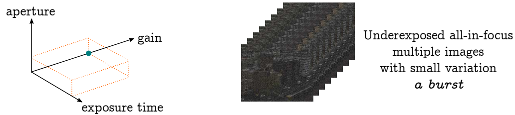
Figure 2.9 – (left) Burst photography captures all-in-focus images over small exposure time with high gain to overcome imaging trade-offs. (right) An example of a single burst of images: multiple images with high overlap and small exposure.
