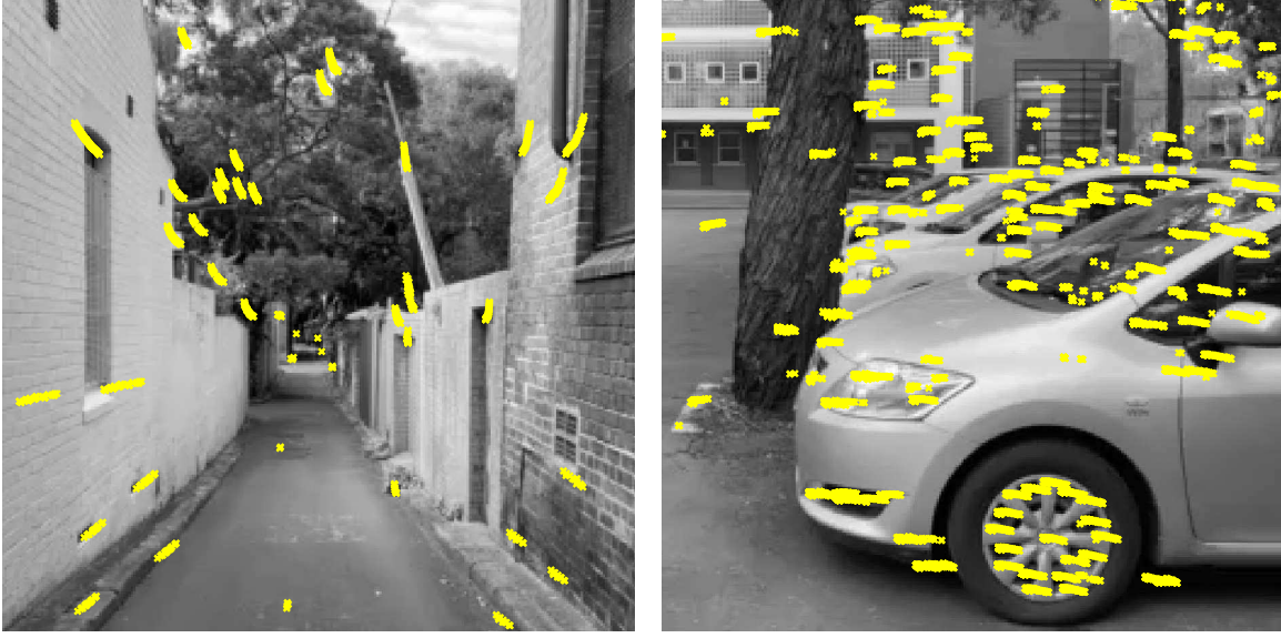
Figure 4.3 – (left): In 3D scenes under general 6-degree of freedom (DOF) platform motion, features in a burst exhibit apparent motion that is well approximated by line segments, even under platform rotation; (right): In the special case of a platform moving orthogonal to the principal axis of the camera, the apparent motion follows parallel line segments. We exploit these observations to search either 2D or 1D spaces of linear apparent motion to detect BuFF features.
