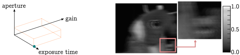
Figure 2.6 – Capturing an image at night with long exposure while keeping the other camera parameters minimum allows more signal, but introduces motion blur. (Contrast-adjusted image for visualisation)
