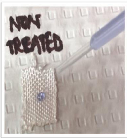
Figure A4 Hydrophilicity experiment of untreated & PIII treated UHMWPE fabric.
