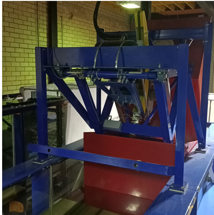
FIGURE 3.4. Photo of the piston-type wave paddle, as installed at the wave flume and controlled by the Njord runtime engine software.
