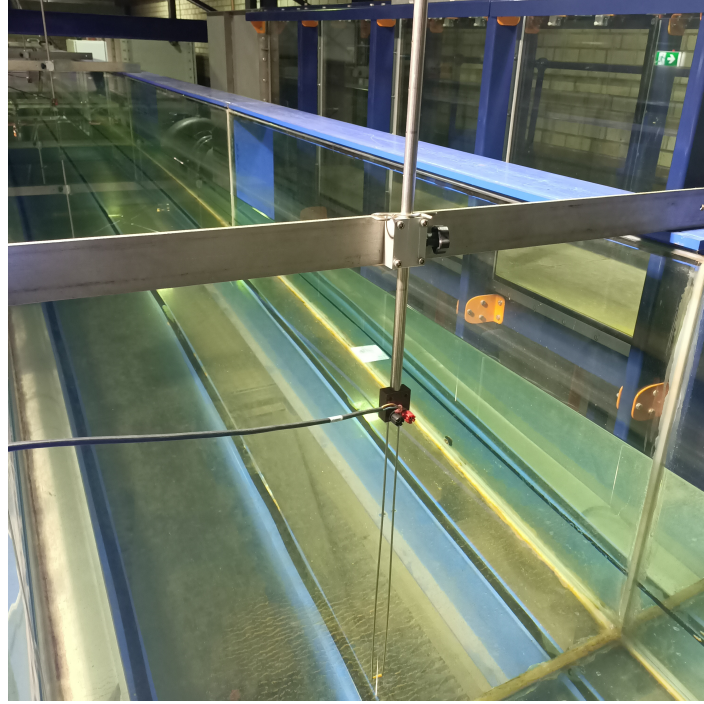
FIGURE 3.3. Photo of a resistive wave gauge installed at the wave flume. The bottom u-shaped long conductive metal is partly immersed to measure the water level. The cable extended from the wave gauge transfers the electric current signal to the USB fast hub interface and eventually to the data capture file.
