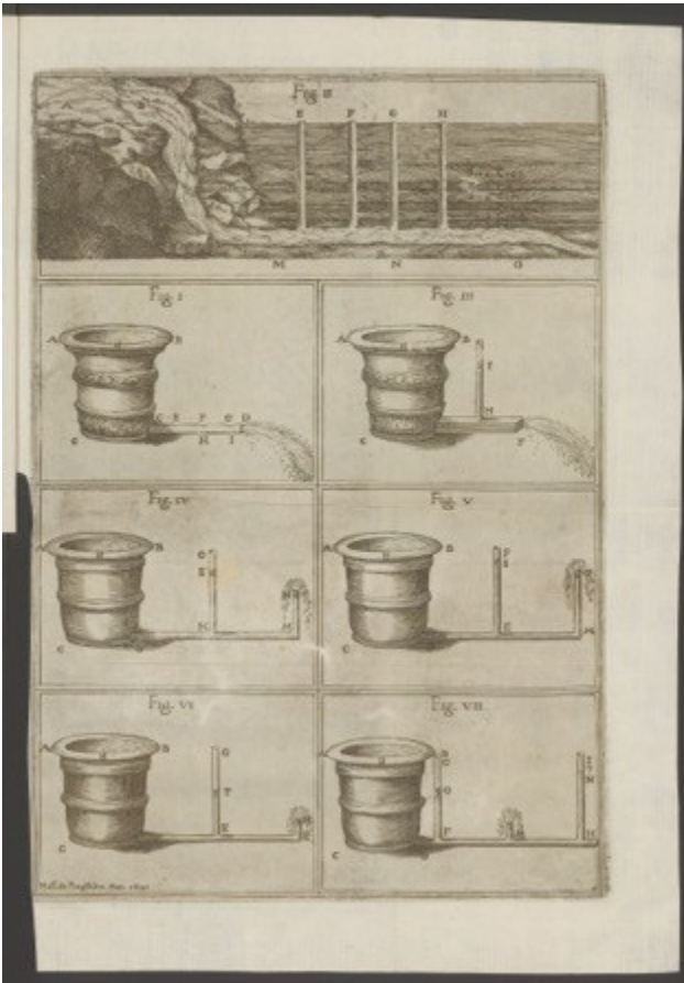
Figure 10: Wells bored through Modena's strata into its water supply (Fig. II), and hydrostatic experiments below, in Ramazzini's De fontium mutinensium (1691). Credit: Zentralbibliothek Zürich, NG 420,4, Public Domain Mark.
