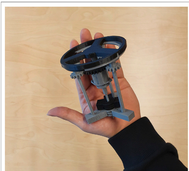
FIGURE 7 | A proposed control unit sizing and learning poly(lactic acid) (PLA) prototype. This control unit was prototyped to show preliminary feasibility and identify learning points in preparation for more extensive metal prototyping. It is the complete triplicate prototype for the single subunit (one third) mechanism shown in Supplementary Video S3 . Each subunit controls three rods and the three subunits are added together in a wheel-and-spoke fashion with 120 degrees between each subunit. The complete control unit was designed to control up to nine rods in a narrow-diameter (2 cm) keyhole surgical instrument such as the one detailed in our preliminary brief research report (Roche et al., 2021b).
