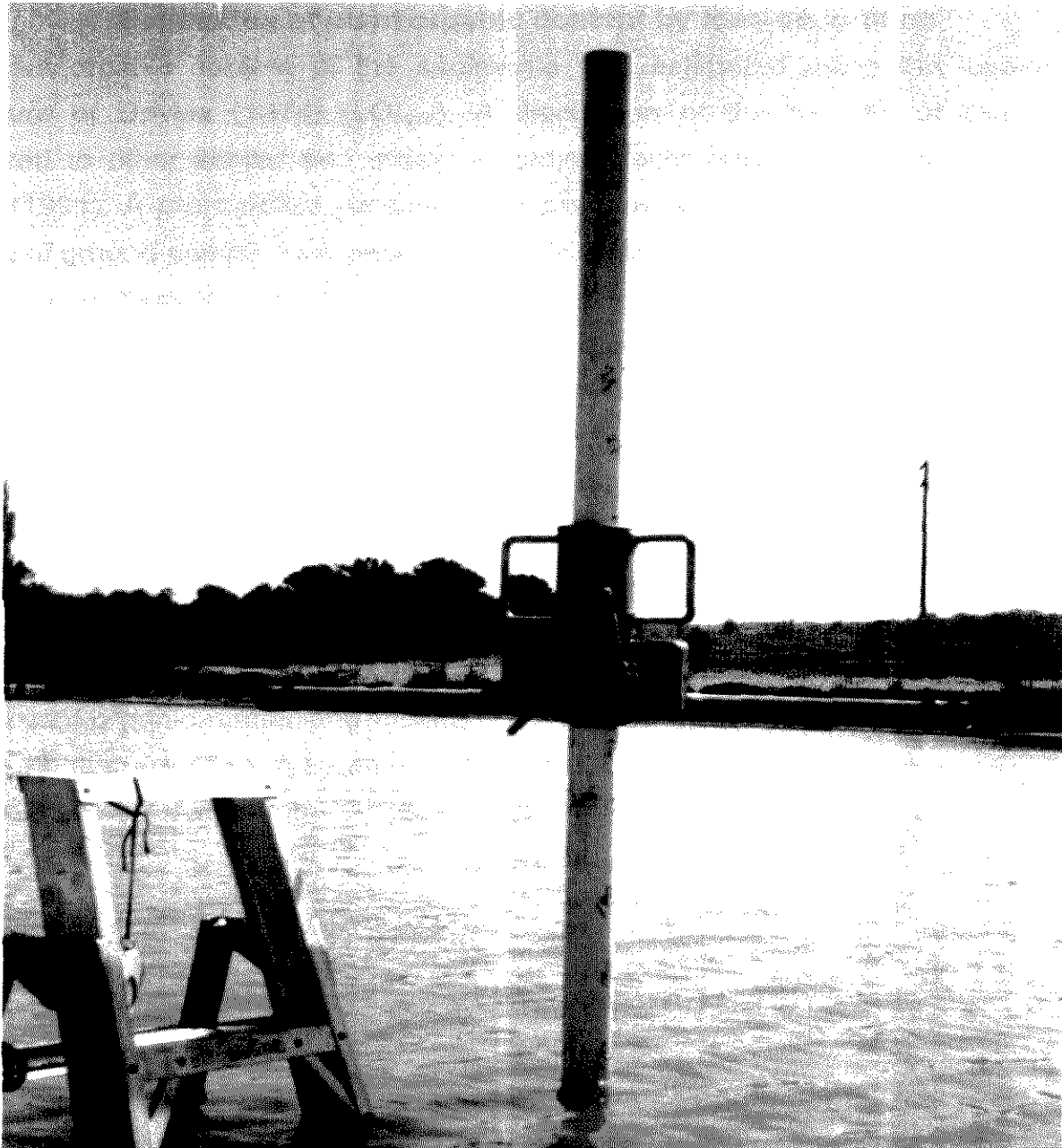
Figure 5.3 Percussion coring along the A-transect using 50 mm PVC tubes, Tocal Homestead Lagoon, 1998.
