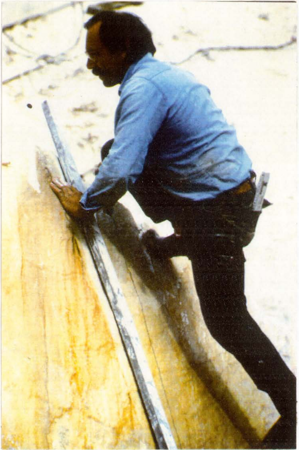
Plate 13. Foreman, Arimante, measuring a block of marble for cutting.
