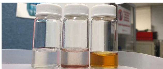
Figure 10. Iodometric titration process (right to left: via containing electrolyte after 30 min reaction, via containing electrolyte after adding Na 2 S 2 O 3 , via containing electrolyte after complete titration).
