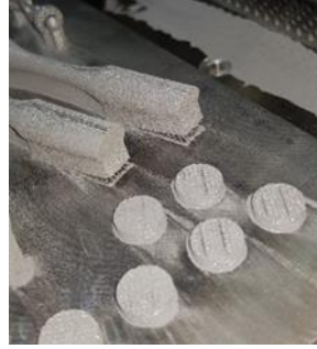
Figure 2-15 Distorted Ti6Al4Va specimens in this study
