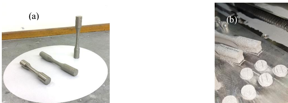
Figure 7-2 (a) Vertical and horizontal SLM and wrought Ti6Al4Va and (b) distorted SLM horizontal specimens
