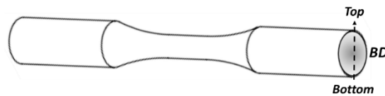
Figure 3-3 Hardness measurement from bottom to top in the built direction, labelled BD
