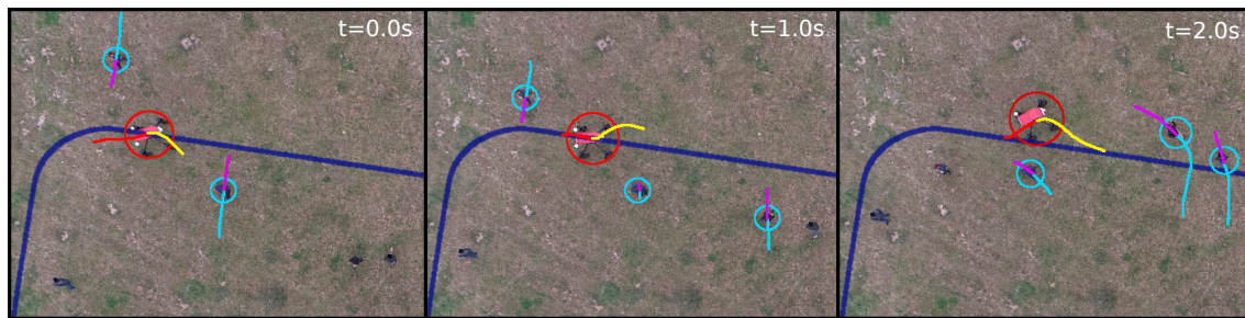
Figure 4.10 – Subsequent time steps to Fig. 4.9 during the crowd interaction trial. The robot’s best path found using the MCTS-GRNN dynamic planner is shown in yellow as it tracks the reference path (dark blue). The mean predicted path of each agent in response to this chosen path is shown in purple. Step 1 shows the robot choosing a path behind the approaching agent. In step 2, when the agent stops rather than following the predicted motion, the robot updates its plan accordingly. In step 3, the robot returns to the reference path, avoiding the new agents. Only agents tracked by the robot each timestep are highlighted.
