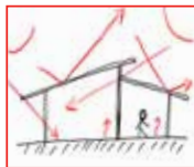
Natural light The shape of roof can let the natural light in therefore save electricity and make people feel more comfortable.
