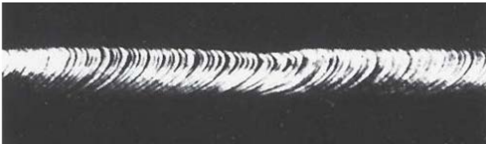
Figure 2.3 Illustration of slip in a single zinc crystal. Modified from [49].
