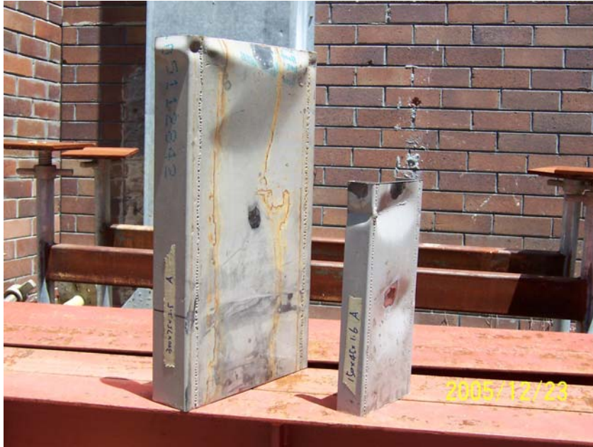
Figure 9. Deformation of Tested Specimens (300×75×2.5 (A) and 150×45×1.6 (A))
