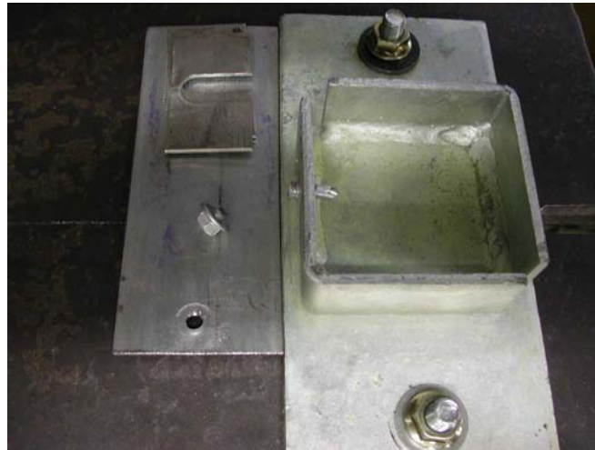
Figure 6: Single screw test after failure
