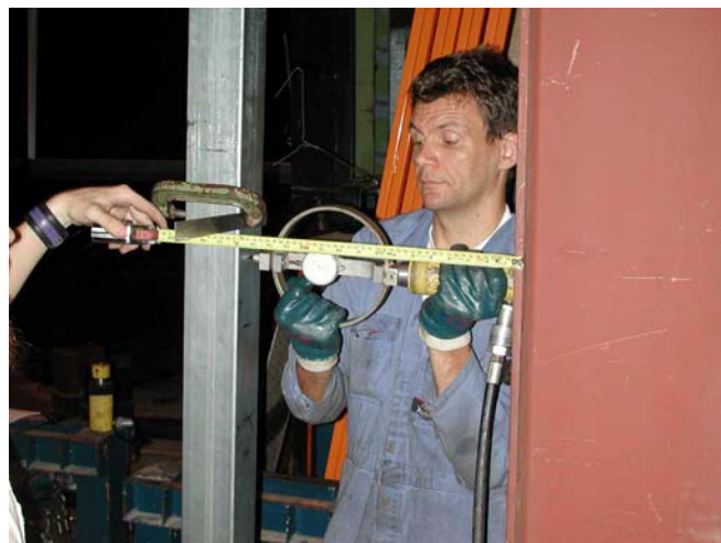
Figure 9: Cantilever test setup
