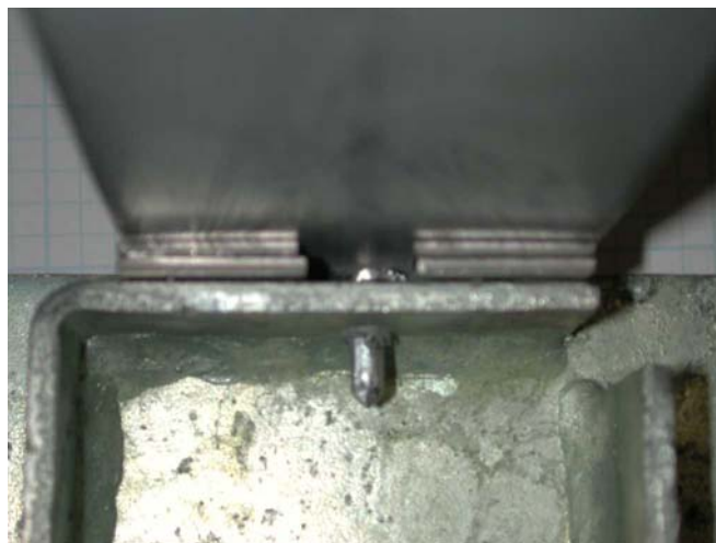
Figure 3: Single screw inserted with packing
