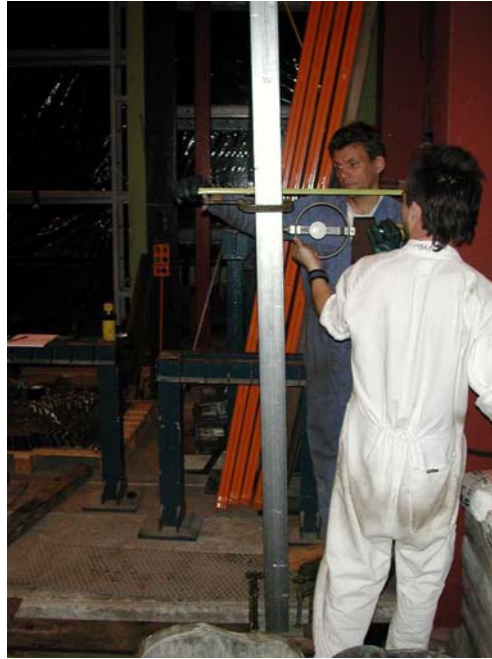
Figure 10: Cantilever test near failure
