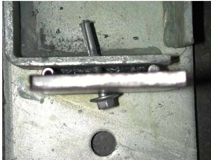
Figure 8: Single screw inserted at an angle of approximately 20°
