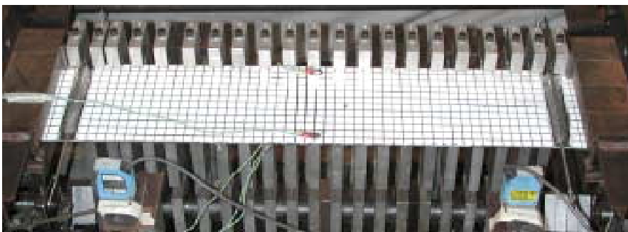
Figure 8: (a) End bearings and fingers provide three-sided simple support (b) Laser device and target
