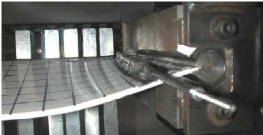
Figure 11: Limit of end rotation due to contact of specimen and bearing block
