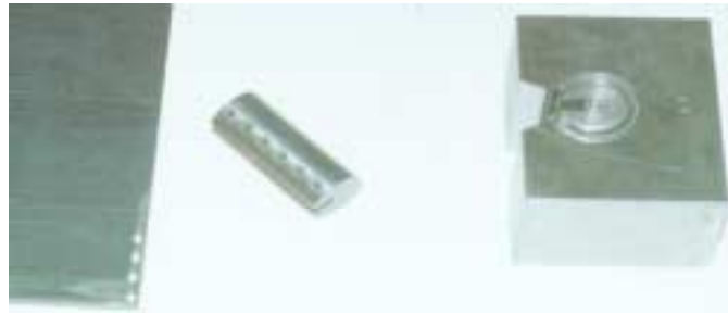
Figure 6: Loaded edge of a plate specimen, rod segment and end bearing
