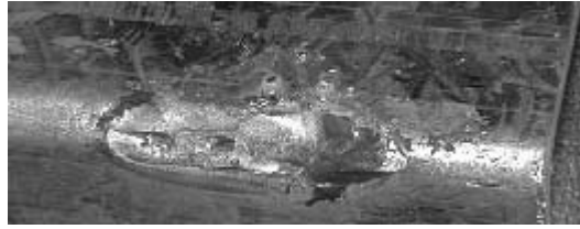
Fig. 10 Fracture of flare-bevel welds in 3.0-mm G450 sheet steel
