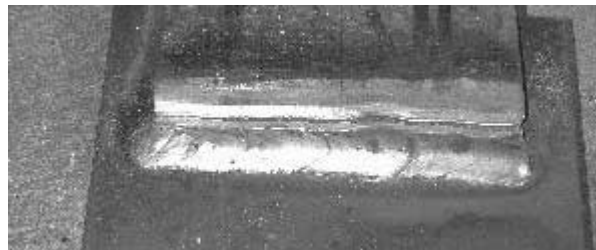
Fig. II.1 Fillet weld in 3.0-mm sheet steel produced by Fabricator B
