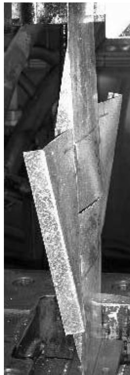
Fig. 18 Gross deformation of 1.5-mm specimen
