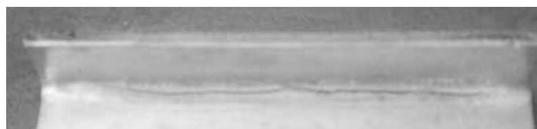
Fig. 7 HAZ failure in 3.0-mm G450 sheet steel
