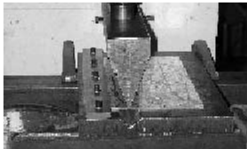
Fig. 4 Sheet steel specimen about to be brake-pressed
