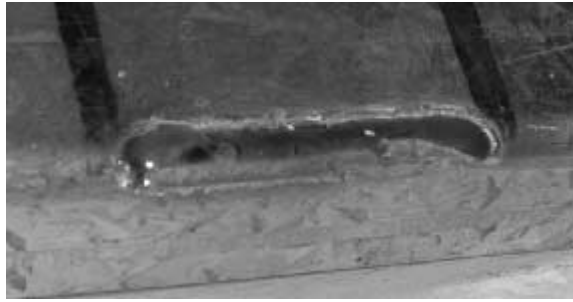
Fig. 19 Weld shear failure of flare-vee welded connection in 3.0-mm sheet steel
