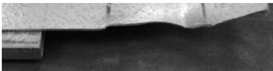
Fig. 7 HAZ failure of double-lap longitudinal fillet welded connection in 1.5-mm sheet steel
