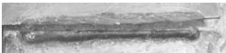
Fig. 15 Weld failure of a single-lap longitudinal fillet welded connection in 3.0-mm sheet steel
