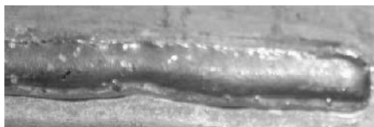
Fig. 11 HAZ failure of a single-lap transverse fillet welded connection in 3.0-mm sheet steel
