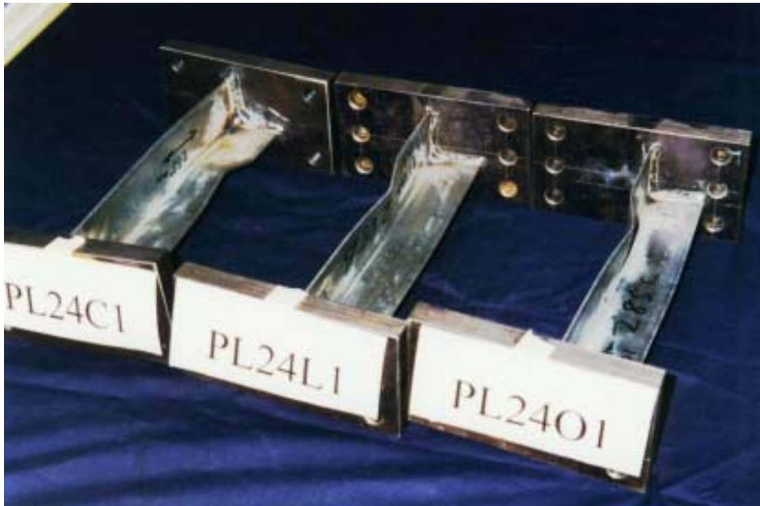
Figure 13: Failure of short specimens (Group 1)
