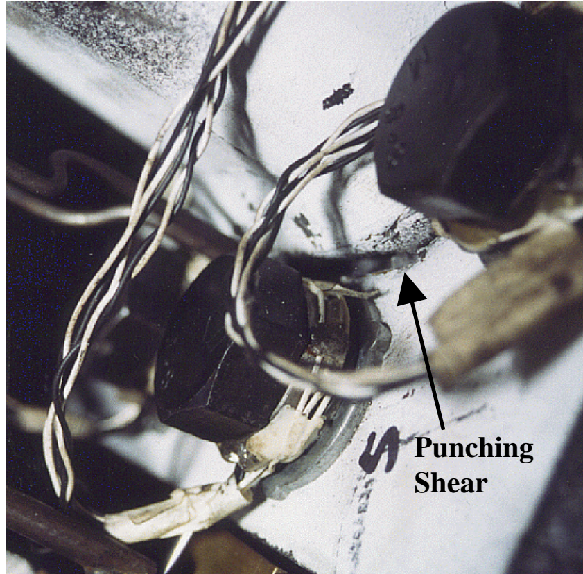
Figure 16 - Plate Punching Shear
