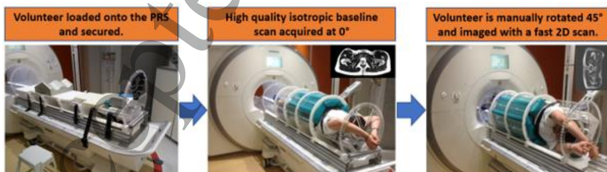
Figure 1: Workflow of the PAROT study. The volunteer was first loaded into the patient rotation system and secured. An isotropic scan was then acquired in the supine (0° rotation) position before being manually adjusted in 45° increments. A faster scan was acquired in the supine (0° rotation) position before being manually adjusted in 45° increments. A faster scan was acquired at each position.
