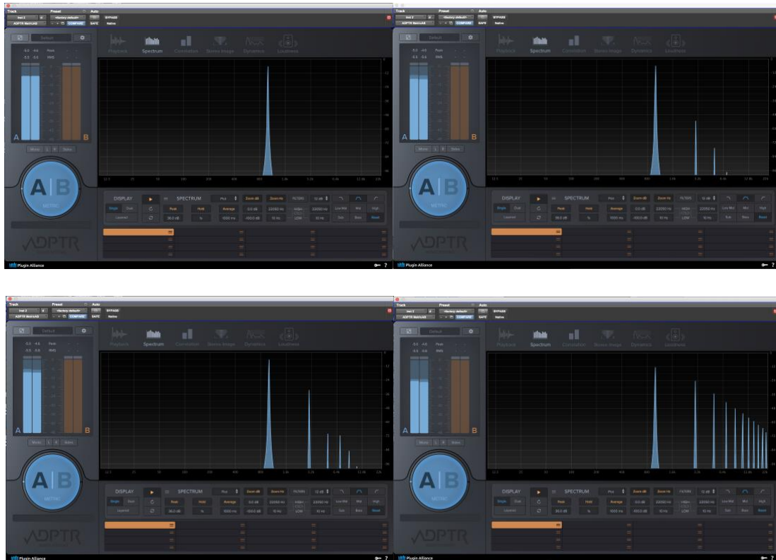
Figure 10. a. Spectral analysis of 1kHz sine wave with J37 plugin bypassed. b. Spectral analysis of 1kHz sine wave with J37 plugin engaged. c. Spectral analysis of 1kHz sine wave with J37 plugin 'saturation' parameter set to halfway. d. Spectral analysis of 1kHz sine wave with J37 plugin 'saturation' parameter set to full.
