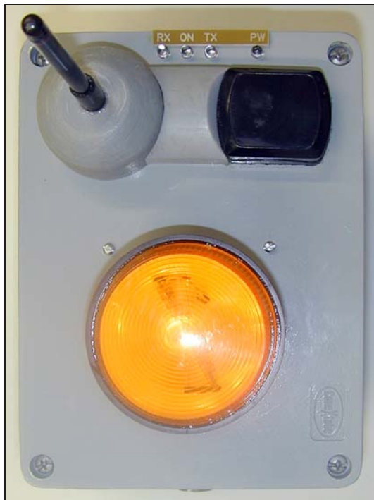
Figure 2.12: Light vehicle node CPS — Light vehicle nodes also have a GPS built in. The RF antenna can be seen on the upper left corner of the node. These nodes are mounted on the roof of the vehicle cabin.
