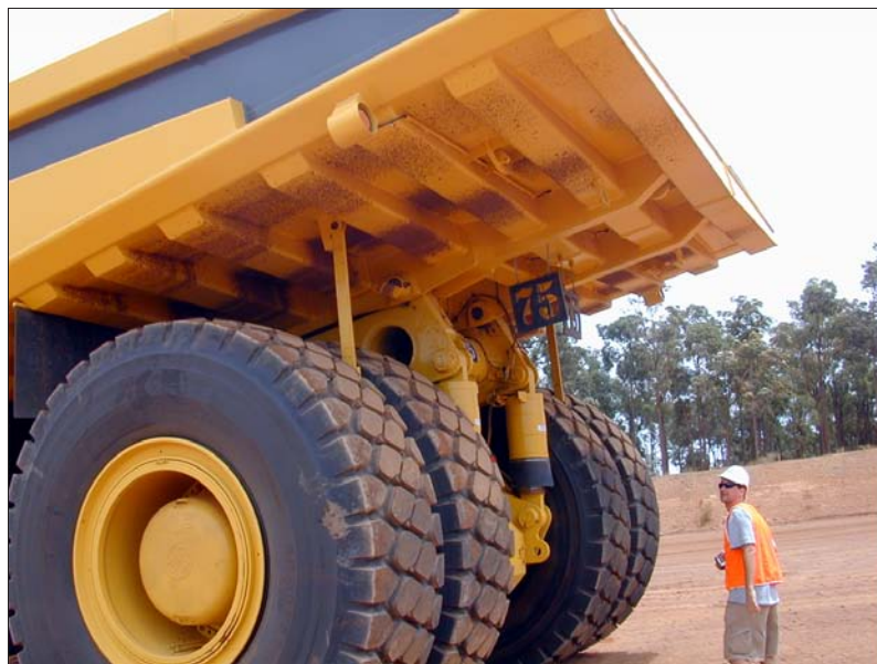
Figure 2.5: Personnel operating in a blind spot — This picture clearly shows how a truck driver sitting the cabin cannot see the person behind the truck.
