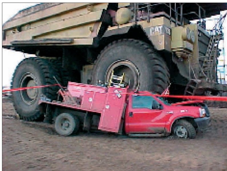
Figure 2.6: Accident in a mine (1 st example) — A truck ran accidentally over a light vehicle. The driver of the truck cannot see the vehicle from the cab. The picture is taken from [2].
