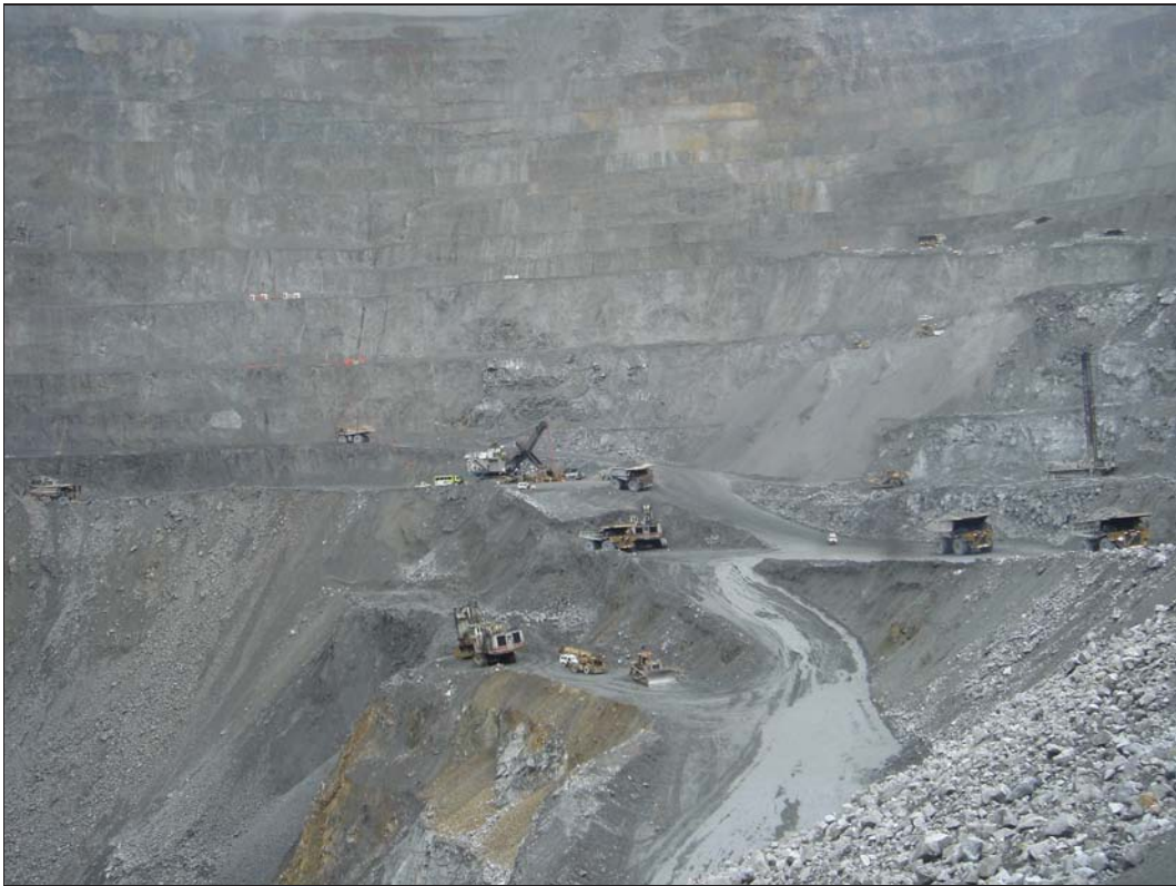
Figure 2.3: Complex machine interactions in a mine — A lot of mobile equipment operates in larger mines alongside each other and has to interact with each other. To further complicate the situation, drivers can leave their vehicles and become exposed to the larger machines. Note that the small white dots in the picture are light vehicles.
