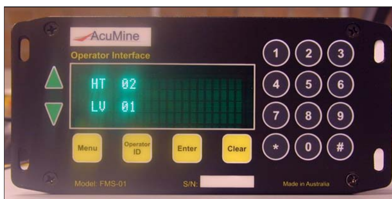
Figure 2.13: Light vehicle operator interface CPS — Using a simple text based interface the number of haul trucks (HT) and light vehicles (LV) in close proximity can be reported to the driver of a light vehicle.
