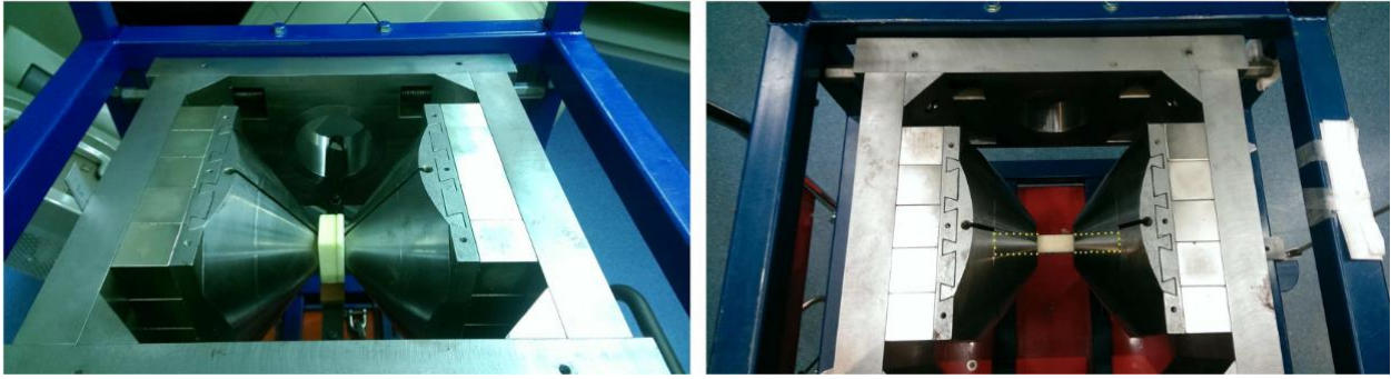
Fig. 1. Experimental setup. Left: experiment 1 contains a 5 \times 7.5 \times 3 \text{ cm}^3 lung phantom with film insert. Right: Experiment 2 contains a 2.4 \times 2.4 \times 15 \text{ cm}^3 lung phantom with film placed along the beam central axis and inside the cone tip holes. An outline of the lung phantom is shown superimposed.
