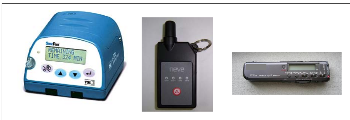
Figure 2: The portable pollution monitor (left), GPS logger (middle) and digital voice recorder (right) used in the study
