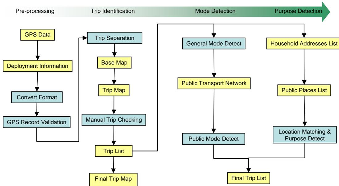
Figure 3: GPS data processing procedure
