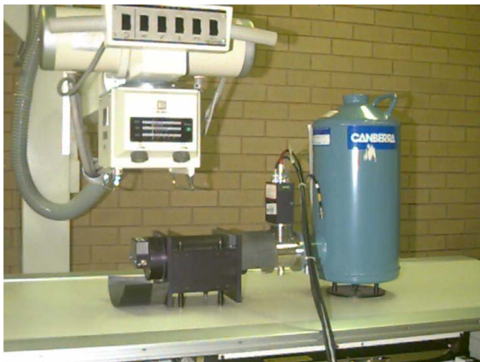
Figure 3.8 Compton spectrometer and its relationship to the x-ray tube and HPGe. Lead sheeting is distal to the spectrometer to reduce backscatter
