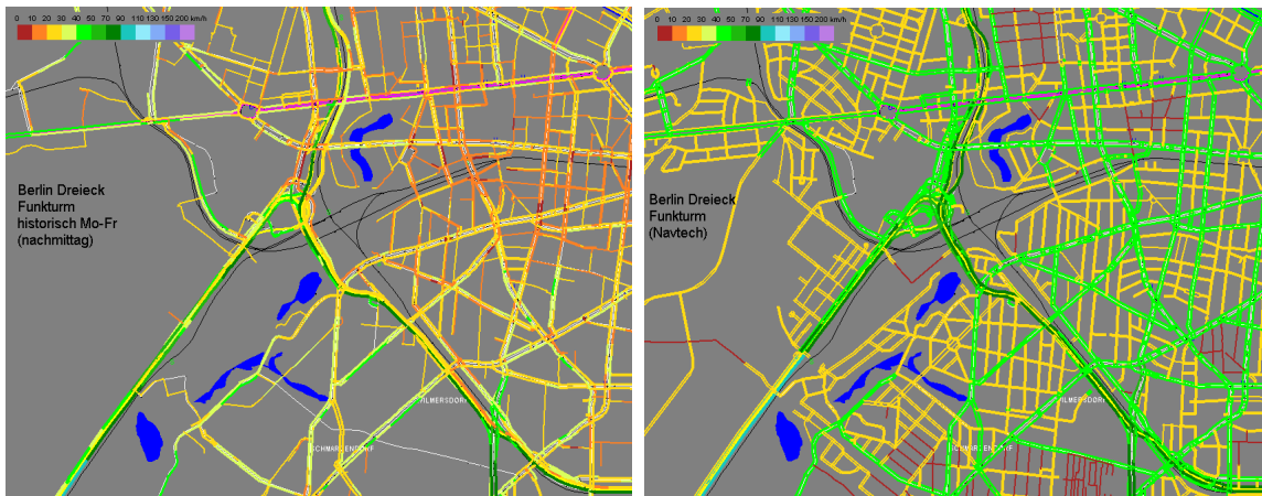
Figure 4: Berlin, historical measurements by Taxi-FCD for the afternoon rush-hour (left), Navtech ® Speed types (right)
