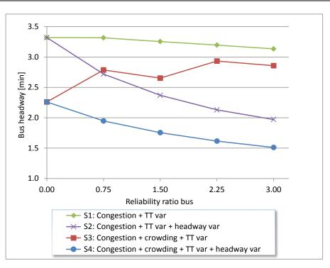
Figure 5: Optimal bus headway
