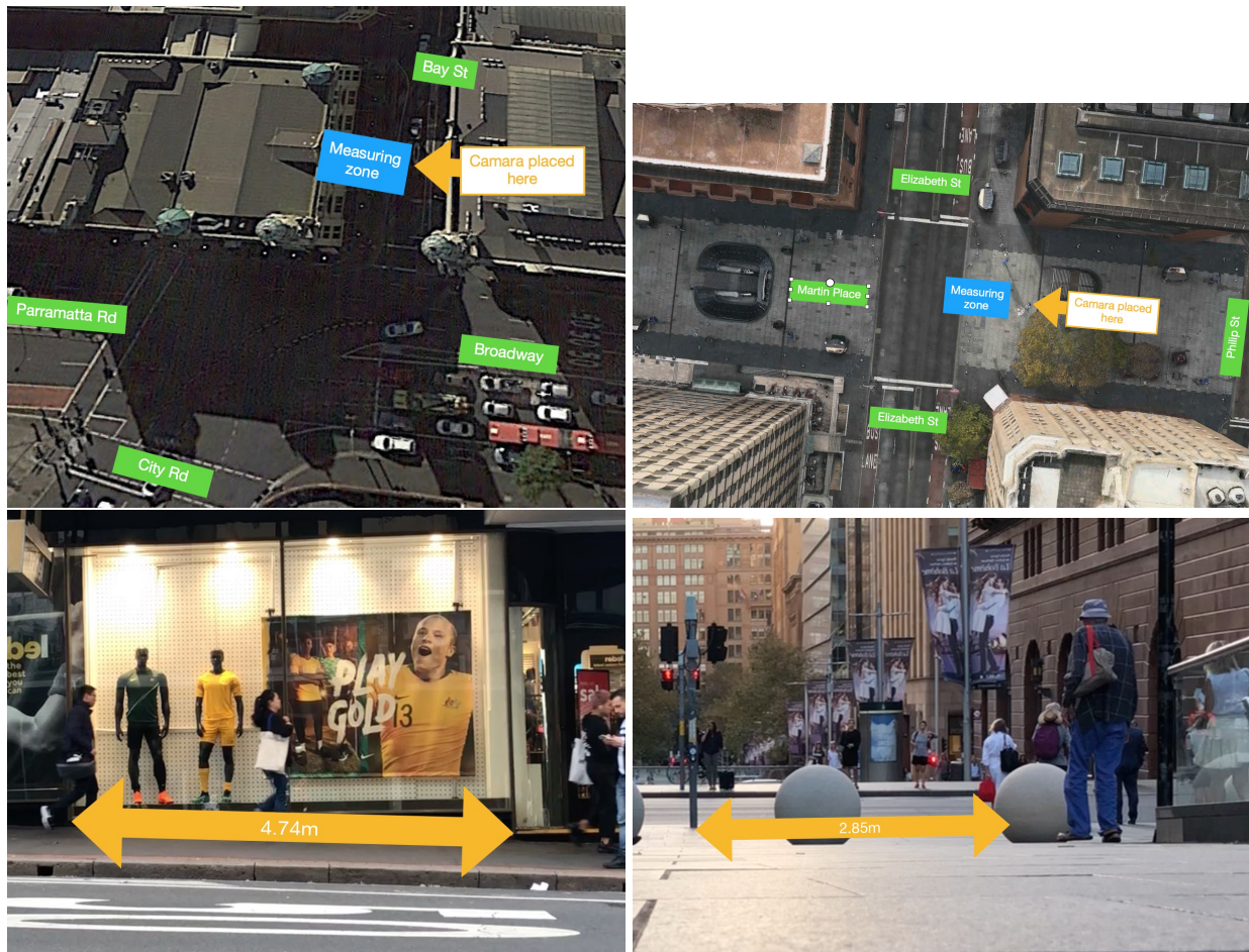
FIGURE 2 Sites 2 and 3: (a) Camera layout Bay St (Site 2) (b) Camera layout Martin Place (Site 3) (c) Measuring zone Bay St (Site 2) (d) Measuring zone Martin Place (Site 3)
