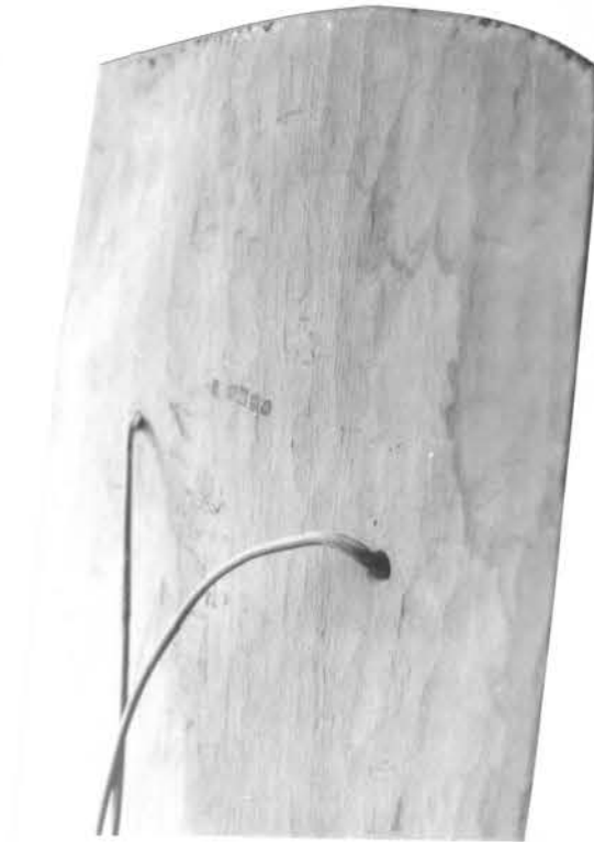
PLATE 26. — Markings typical of use of steel axe
