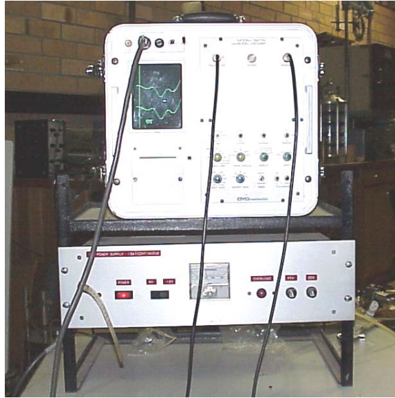
Figure 5.50 The ultrasonic device used for measuring shear modulus of intact shales
