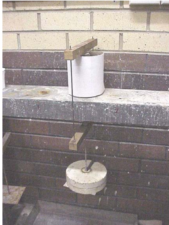
Figure 5.3 Consolidation of the reconstituted specimen under dead weight
