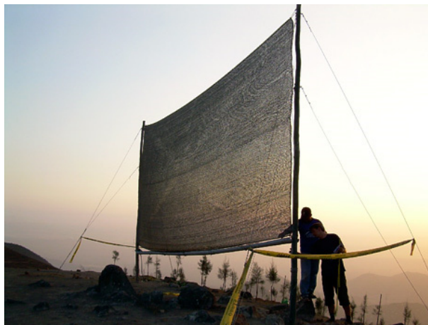
Figure 1.11: Mesh structure used for fog water collection in Bellavista, Peru. 135
