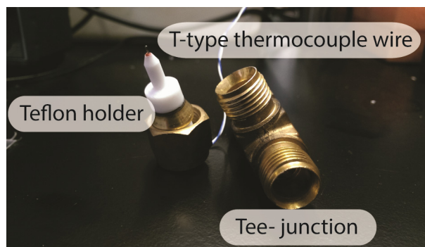
Figure 3.7: Photograph of the components of the thermocouple housing and the Teflon thermocouple holder.
