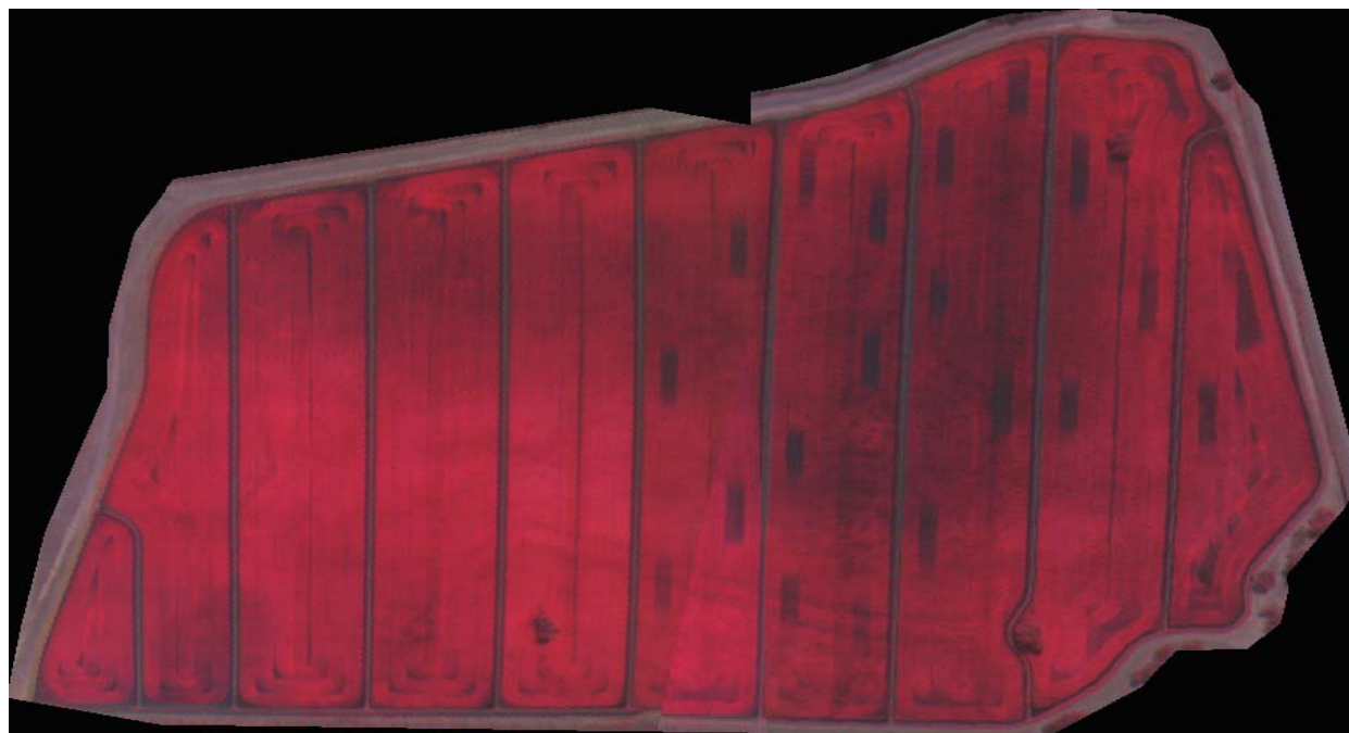
Fig. 9. False infrared colour image of a rice paddock at Jerilderie in February 2002. N fertiliser was applied at sowing at the rate of 120 kgN/ha across the paddock, except in small areas shown as dark strips in the image. The large generally dark area in the right-central part of the paddock is a low-growth area where the topsoil was cut during levelling.
