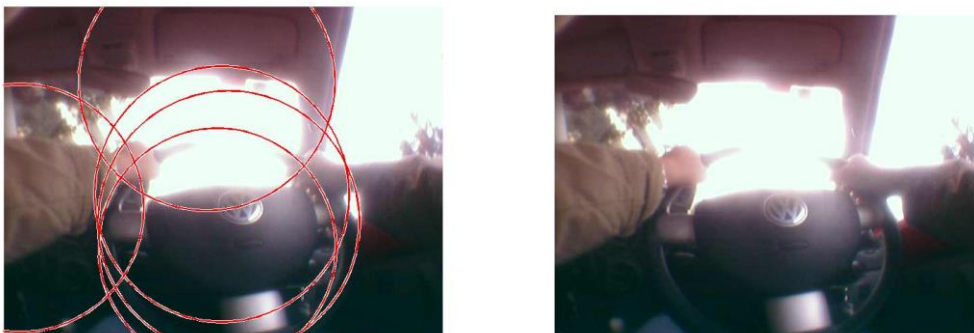
Figure 4.12 Circle Detection for Different Values of Sensitivity
