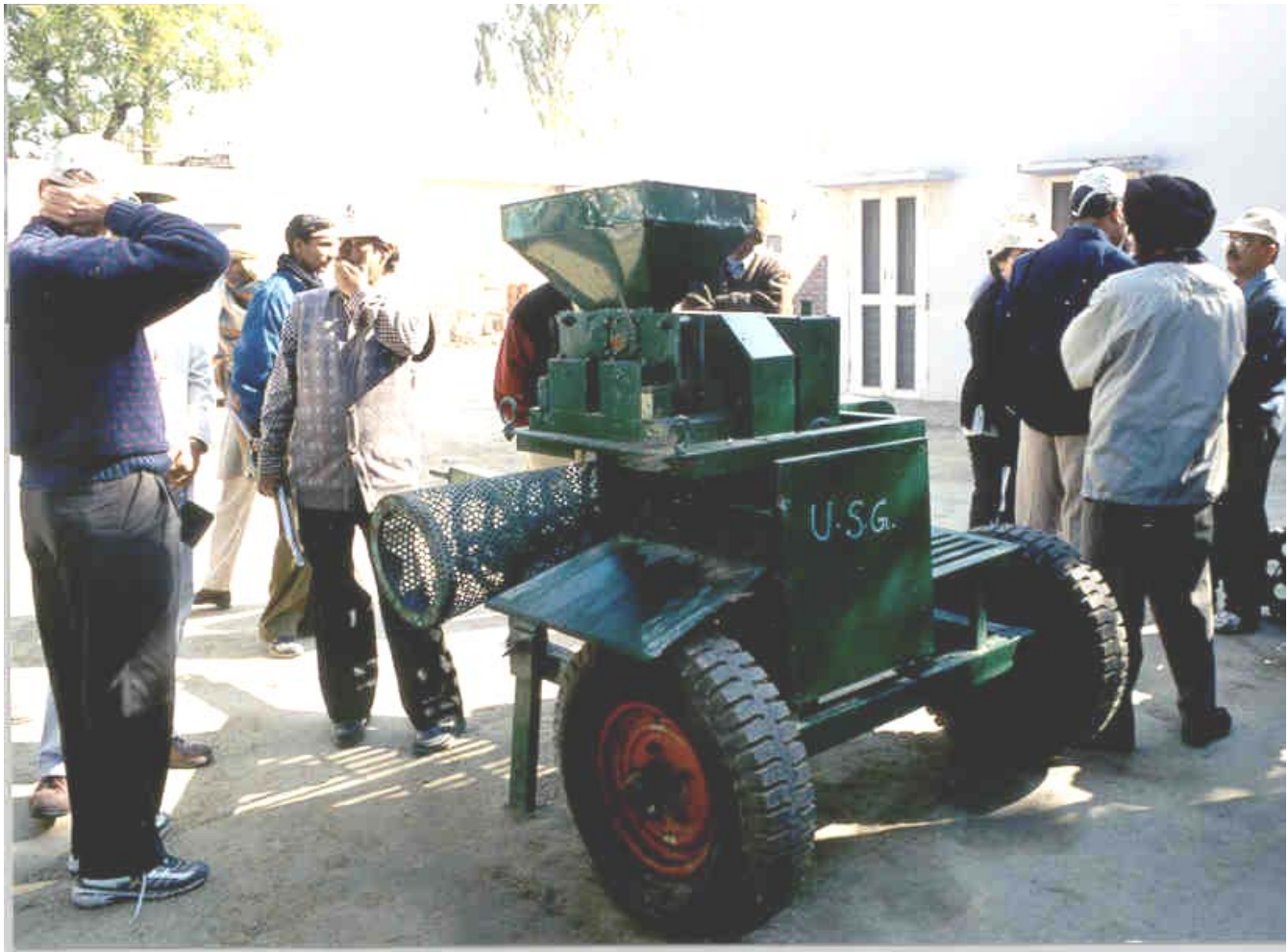
Photo 2. Bangladeshi supergranule making machine modified by the Rice Wheat Consortium for greater portability (wheels, powered by PTO) and to make round granules.
