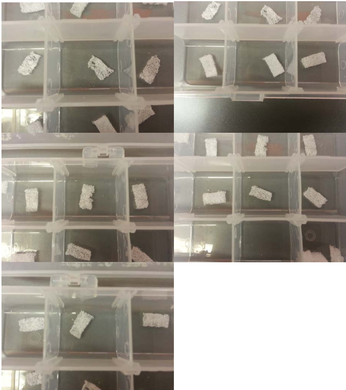
From top left to bottom right: chemically etched microspheres on scaffold, CAP infused scaffolds, Intact microspheres on scaffolds, Negative control, and Positive control.
