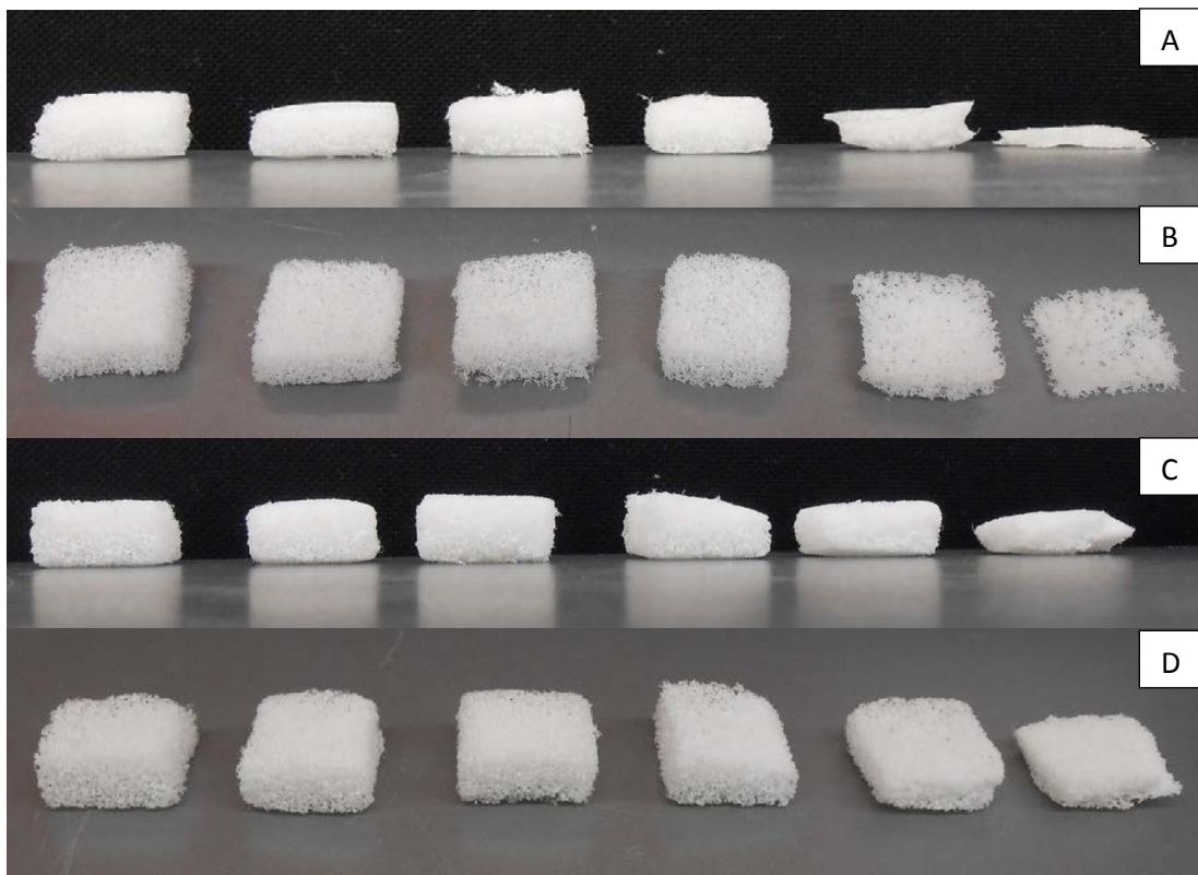
Figure 5-3: Scaffold temperature damage photographs. Images A and B shows plain scaffold temperature damage over 5 minutes and images C and D shows Q-cell coated scaffold thermal damage over 5 minutes. Time points from left to right are 0, 1, 2, 3, 4 and 5 minutes.
