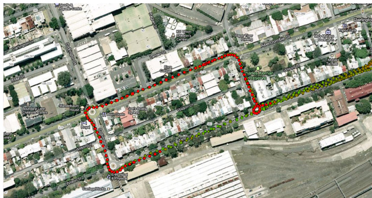
Figure 2.3 – Dead reckoning in a GPS outage. During the outage period of GPS signal (red dots in the figure), the vehicle is still capable of keeping self-localised using the on-board sensors (e.g. compass, accelerometer, speedometer, gyrometer) and route information on the map.
