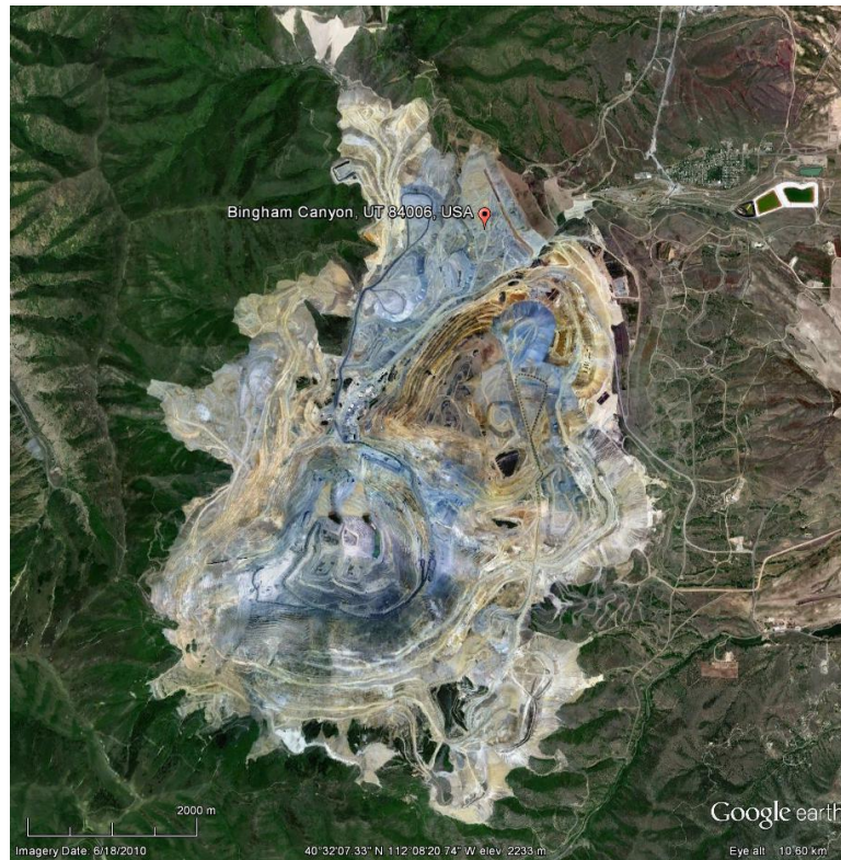
Figure 1.1 – The Bingham Canyon Mine, Salt Lake City, Utah, United States, the deepest open-pit mine in the world. Over 1.21 km deep and 4 km wide, the pit is reported as the world’s largest man-made excavation [170].
