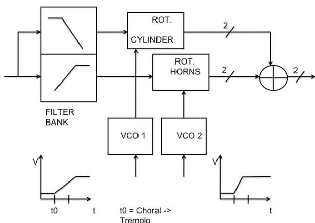
Figure 3. Rotary Speaker Simulation [1]
