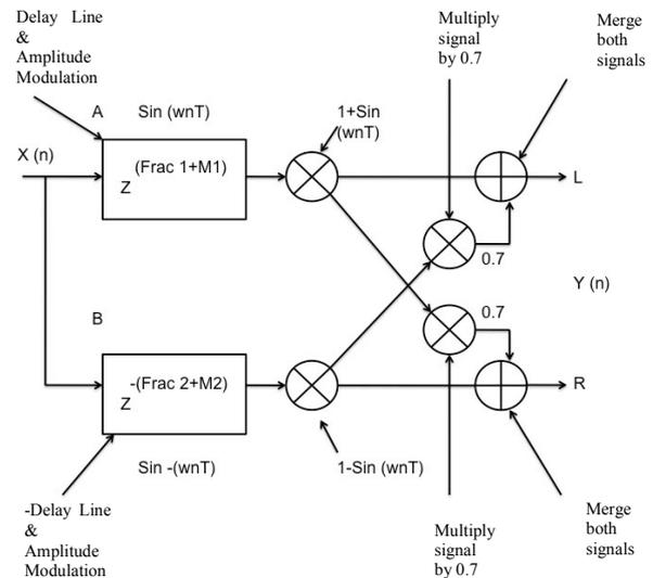
Figure 1. Simulation of rotating speakers [1]
