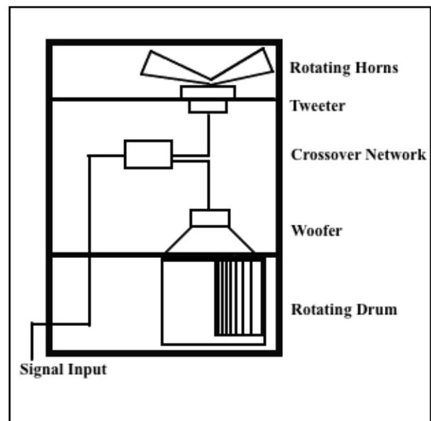
Figure 1. *The analogue two-driver rotary loudspeaker to be simulated with ad DSP algorithm.*
