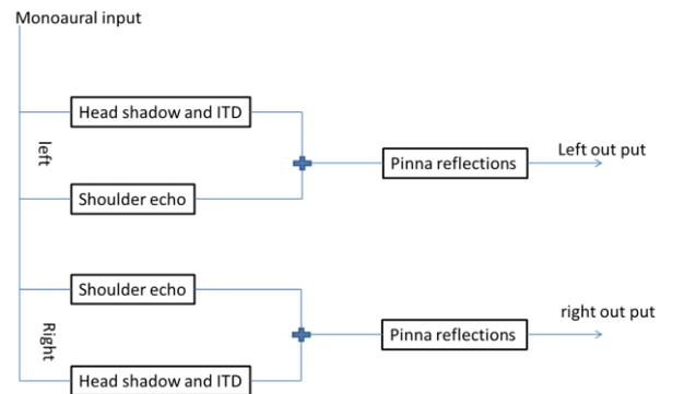
Figure 5 structural model of pinna-head-torso system
