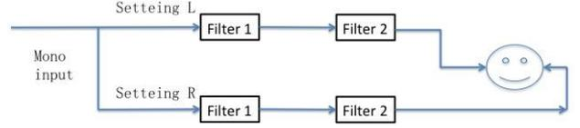
Figure 4 signal process figure of stimulate head shadow and ITD
