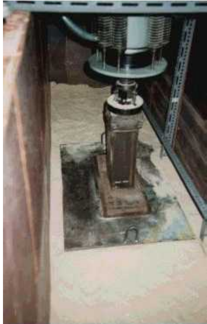
Figure 4-5. Large plate loading (600 x 900 mm, simulating trafficked light pavement)
