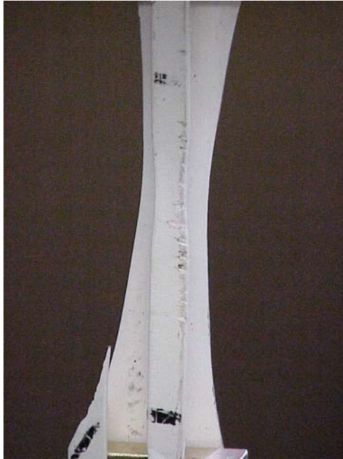
Front view of specimen 1 showing necking of flange
