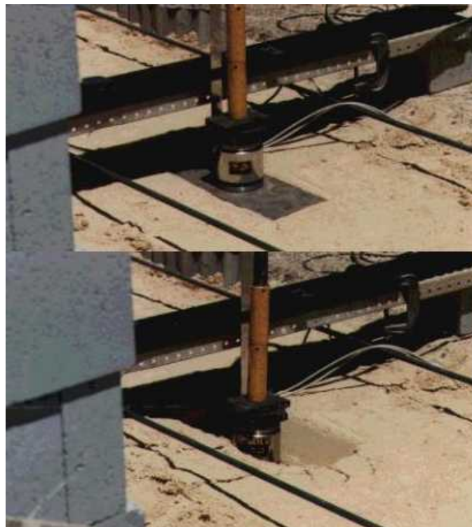
Figure 4-30. Failure of sand upon loading in a field test (0.2 x 0.5 m rigid plate)
