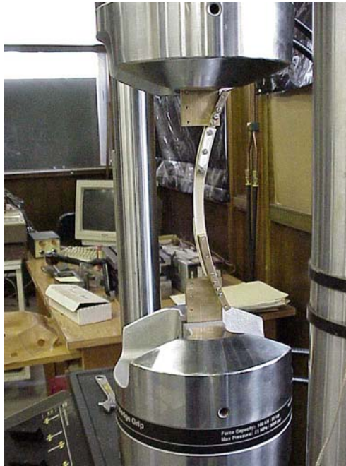
Figure 4-9. Set up of tensile coupon test 1: side view
