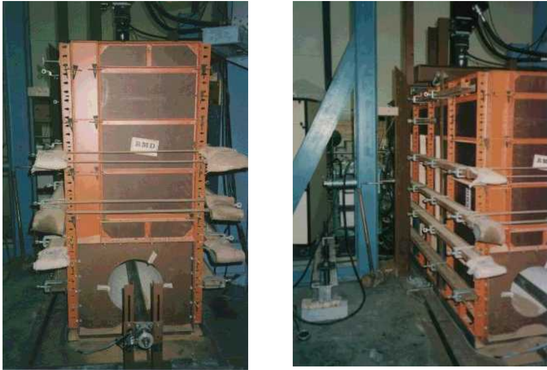
Figure 4-2. The soil box with rotating displacement transducers for measuring internal pipe displacements
