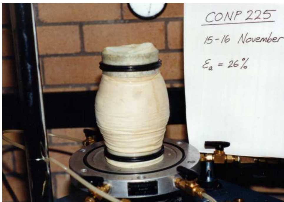
Figure 5-6b. Specimen after a constant pressure test (CONP225, p' = 225 kPa)
