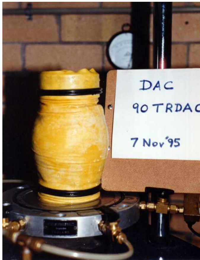
Figure 5-6a. Specimen after a CID triaxial test (90TRDAC, \sigma_3 = 99 kPa)
