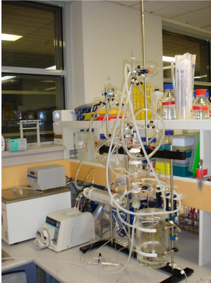
Figure 2.6: Rat Langendorff set up.
