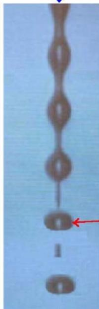
Within the Cytonozzle is the Piezo Crystal. It has a very thin wall between it and the fluid inside the nozzle that creates the stream. An electronic wave is applied at frequencies close to 75khz. This vibration causes the sheath stream to break off into well controlled droplets.
