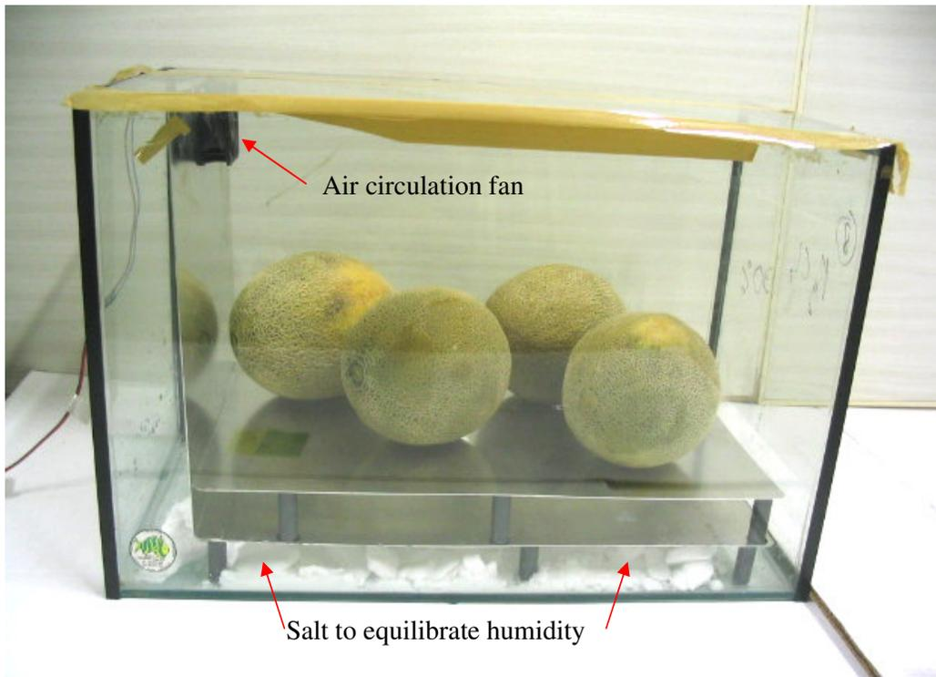
**Plate 3.2.4.1** Humidity chamber for incubation of melons to observe rot development after inoculation with storage pathogens.
