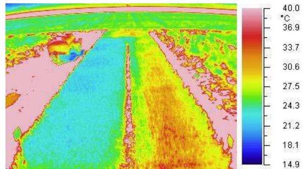
Figure 3. Infrared thermograph of durum wheat Cham 1 plots under irrigated (left) and rain-fed (right) conditions. Photo was taken at 12:00 h.
