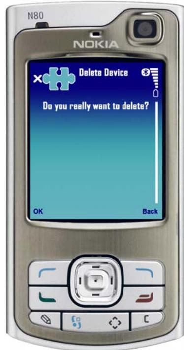
Figure 4.33. If the user does wish to delete a device from the context, a confirmation interface is displayed. The user can select *OK* to proceed with the deletion or *Back* to cancel and return to the *Devices* interface to browse more devices and contexts.
