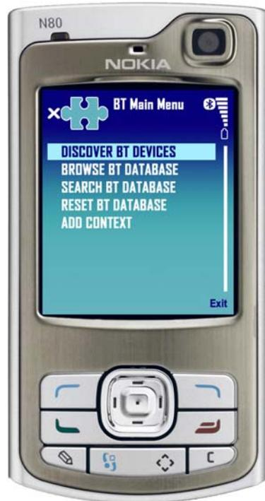
Figure 4.22. The user selects *Discover BT Devices* from the *BT Main Menu* to discover Bluetooth devices and sensors in the area.
