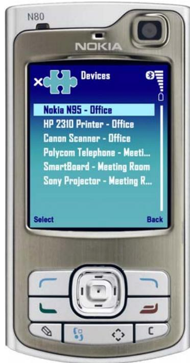
Figure 4.31. The device-friendly names and the context assigned are displayed in the *Devices* interface. The user can choose *Select* to display the individual details of the device or choose *Back* to return to the *BT Main Menu*.
