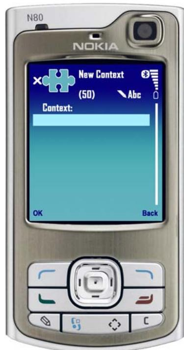
**Figure 4.43.** The user will have to use their mobile device's keypad to manually enter a new context. The context field is restricted to 50 characters, including spacing between the text.
