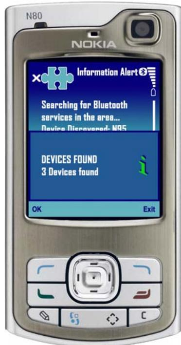
Figure 4.26. When the Bluetooth device and service discovery processes have ended, the `inquiryCompleted` method is called. An *Information Alert* is displayed, showing the total number of *Devices Found*. The user selects *OK* to accept this notification.
