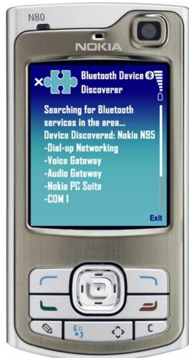
**Figure 4.25.** After the application finds a new service on a Bluetooth device, the *servicesDiscovered* method is called to search for services on the discovered device.
