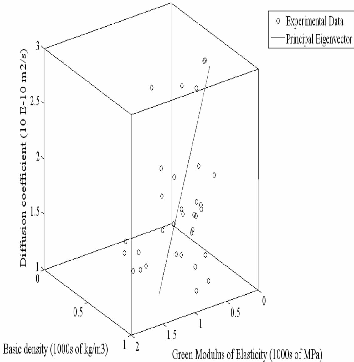
**Figure 6.2.** Three—dimensional plot of the relationship between the diffusion coefficient, the basic density, and the green MOE from the PCA, together with the principal eigenvector (regrowth blackbutt: within—tree test).
