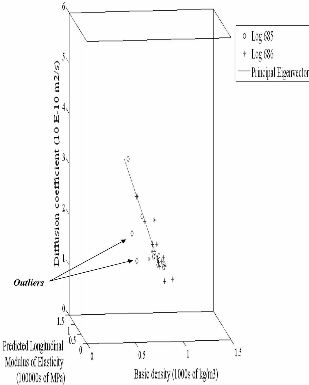
**Figure 6.6.** Three-dimensional plot of basic density, longitudinal modulus of elasticity (predicted using acoustic methods), and diffusion coefficient from Principal Components Analysis (PCA), together with the principal eigenvector (regrowth blackbutt: within— tree test).
