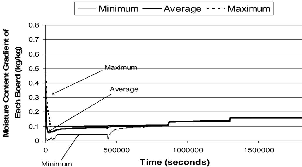
**Figure 6.11.** The minimum, maximum and average moisture content gradient values of all 30 boards, as a function of time, using the drying schedule with temperatures that were 10°C lower than the original drying schedule.
