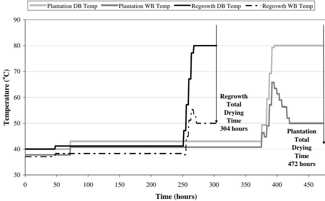
**Figure 6.19.** Optimized drying schedules as a function of time accounting for the variability of regrowth blackbutt boards (between—trees) and the variability of plantation blackbutt boards (within and between—trees).
