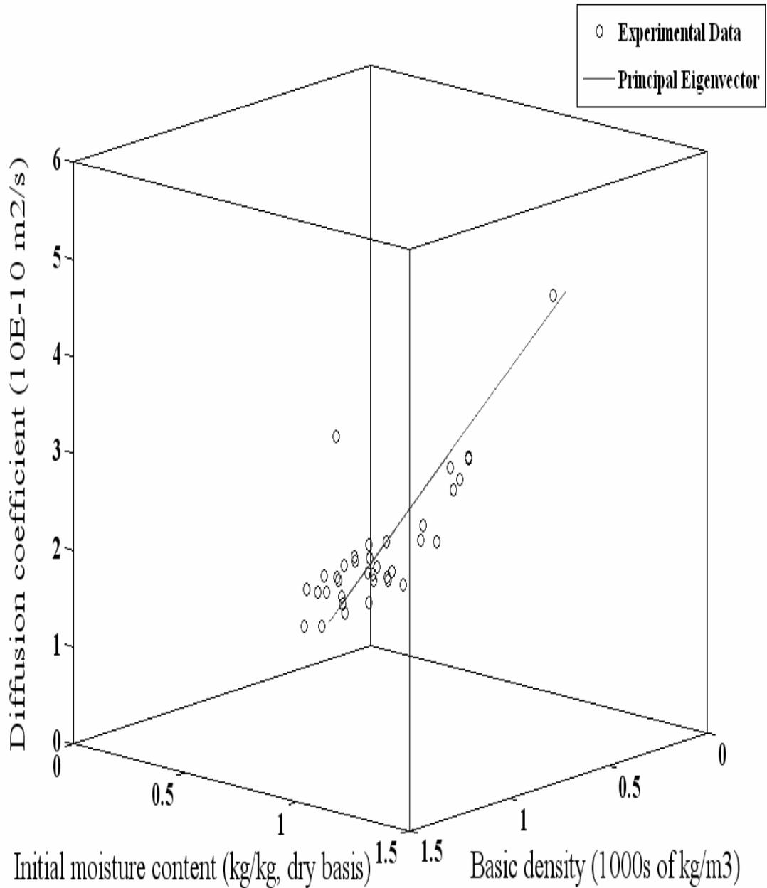
**Figure 6.1.** Three—dimensional plot of the relationship between the diffusion coefficient, the initial moisture content, and the basic density from the PCA, together with the principal eigenvector (regrowth blackbutt: within—tree test).
