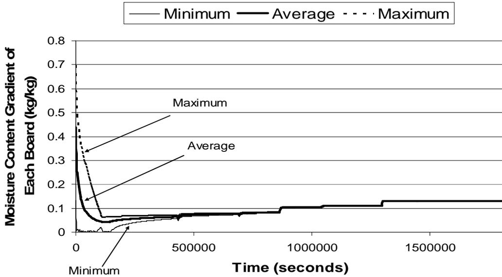
**Figure 6.12.** The minimum, maximum and average moisture content gradient values of all 30 boards as a function of time, using the drying schedule with temperatures that were 10°C higher than the original drying schedule.
