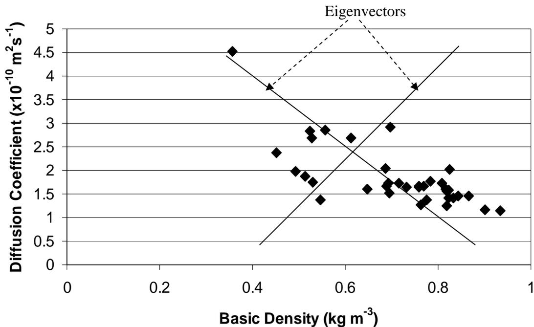
**Figure 6.3.** Experimental data for the within—tree test of regrowth blackbutt and their respective eigenvectors.
