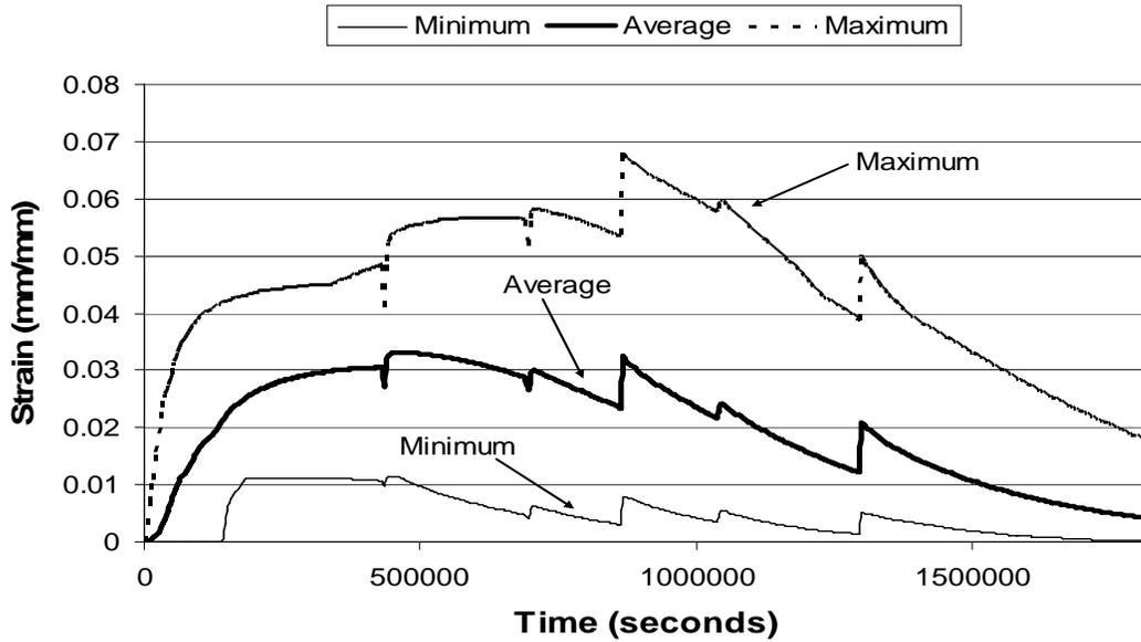
**Figure 6.16.** The minimum, maximum and average strain values of all 30 boards as a function of time, using the drying schedule with temperatures that were 10°C higher than the original drying schedule.
