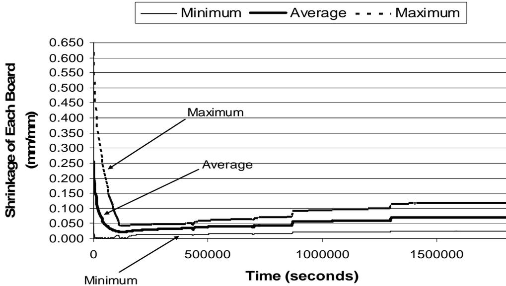
**Figure 6.14.** The minimum, maximum and average shrinkage values of all 30 boards as a function of time, using the drying schedule with temperatures that were 10°C higher than the original drying schedule.
