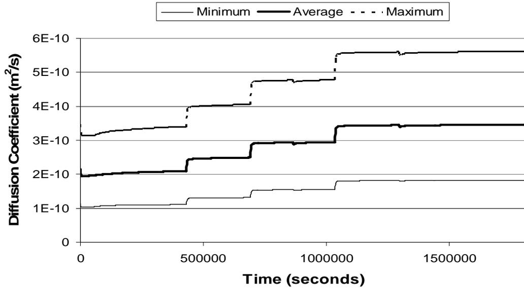
**Figure 6.10.** The minimum, maximum and average diffusion coefficient values of all 30 boards as a function of time, using the drying schedule with temperatures that were 10°C higher than the original drying schedule.
