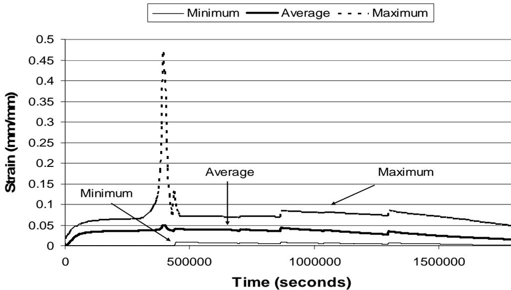
**Figure 6.15.** The minimum, maximum and average strain values of all 30 boards as a function of time, using the drying schedule with temperatures that were 10°C lower than the original drying schedule.
