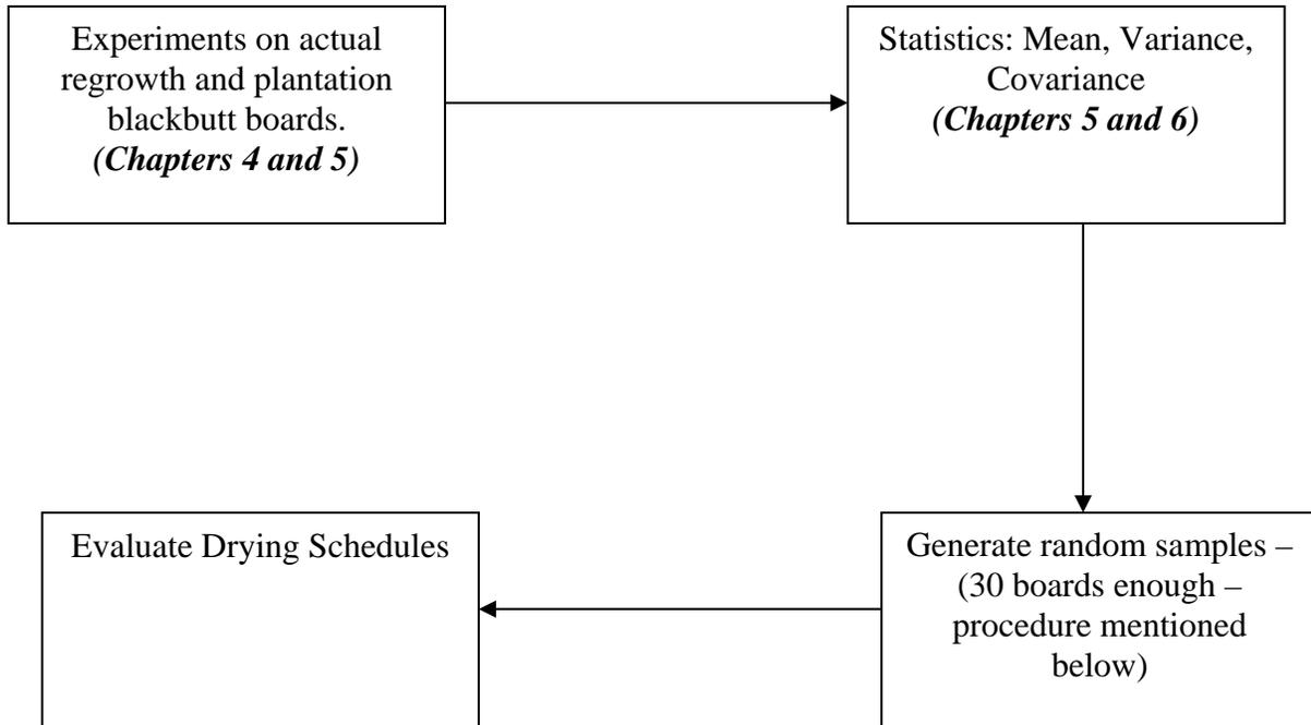
**Figure 6.7.** The overall procedure for evaluating different drying schedules accounting for the variability of regrowth and plantation blackbutt timber.
