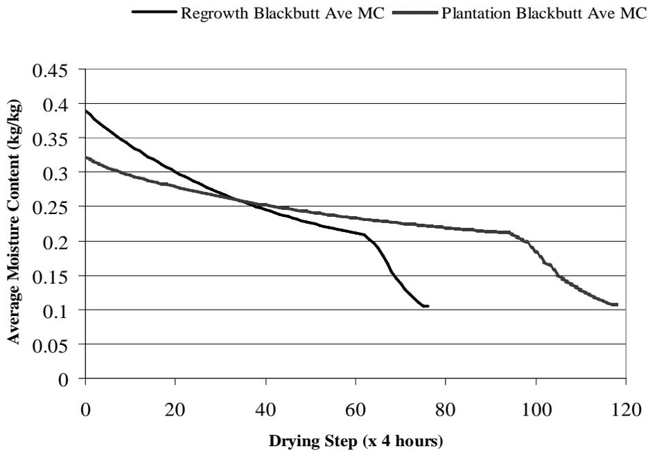
**Figure 6.20.** The predicted average moisture content as a function of time of regrowth and plantation blackbutt timber using the optimization procedure.
