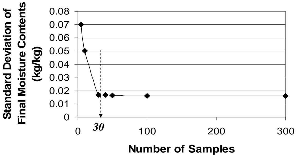
**Figure 6.8.** The dispersion of final moisture contents as a function of the number of samples.
