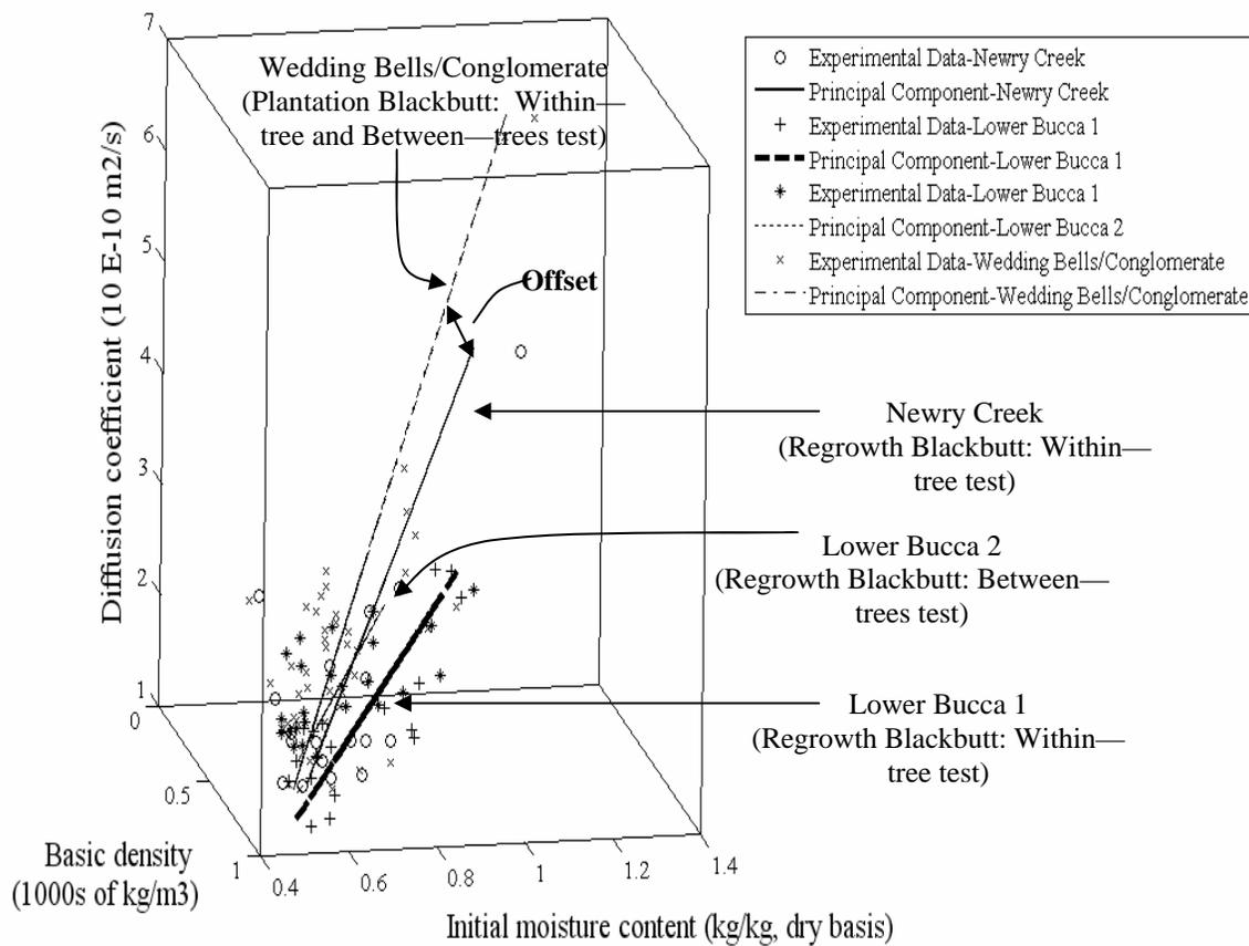
**Figure 6.5.** Three—dimensional plot showing the experimental data and the principal component for each test based on the location where the trees were felled.
