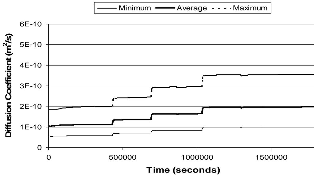
**Figure 6.9.** The minimum, maximum and average diffusion coefficient values of all 30 boards as a function of time, using the drying schedule with temperatures that were 10°C lower than the original drying schedule (regrowth blackbutt timber: within—tree variability).
