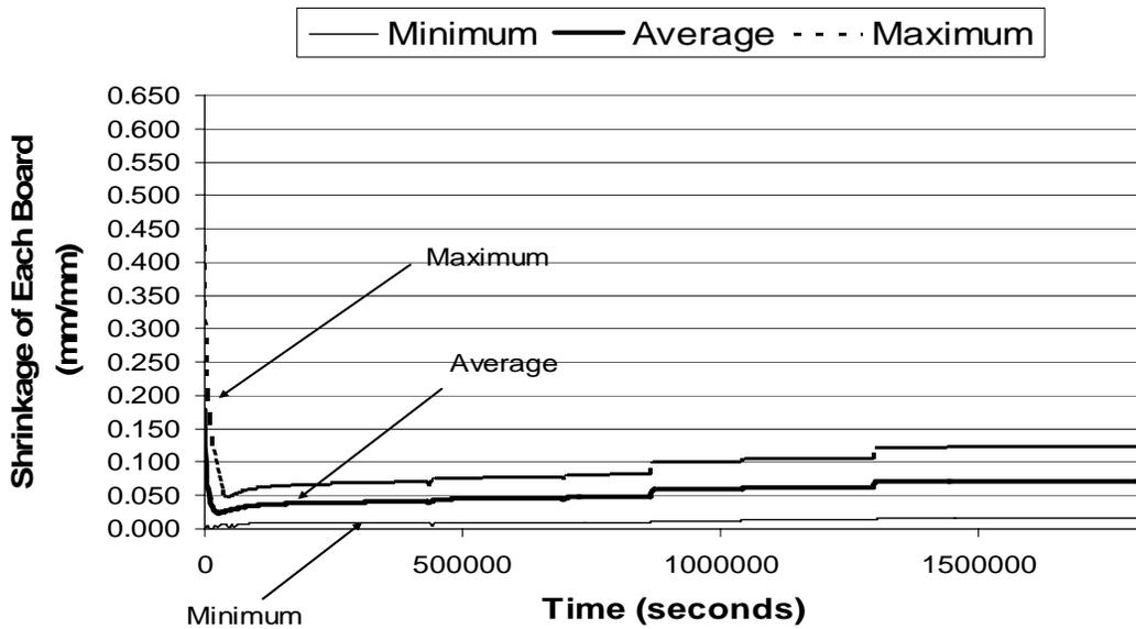
**Figure 6.13.** The minimum, maximum and average shrinkage values of all 30 boards as a function of time, using the drying schedule with temperatures that were 10°C lower than the original drying schedule.
