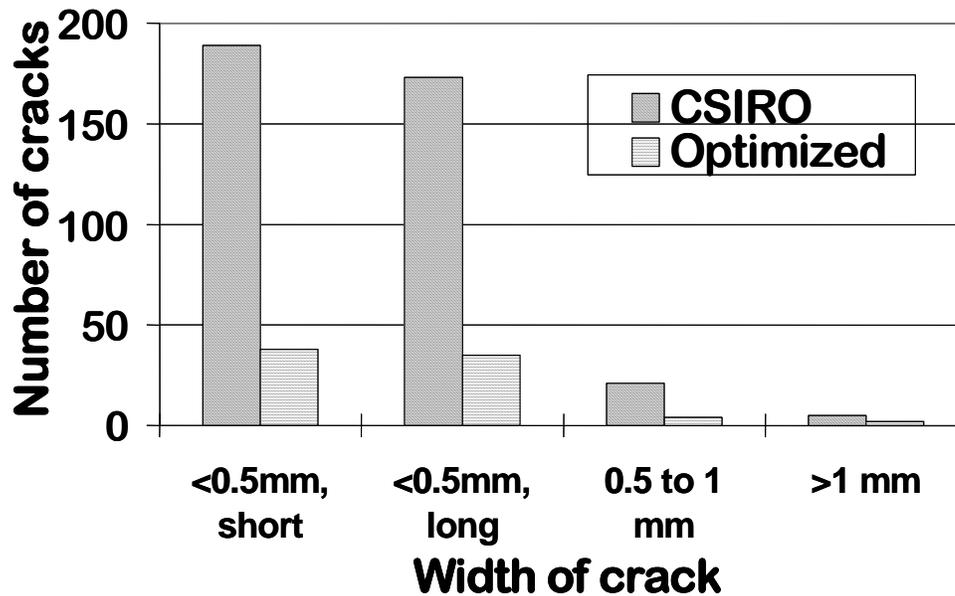
**Figure 2.3.** Comparison of checking obtained from the conventional and optimized drying schedules (Langrish *et al.*, 1997).
