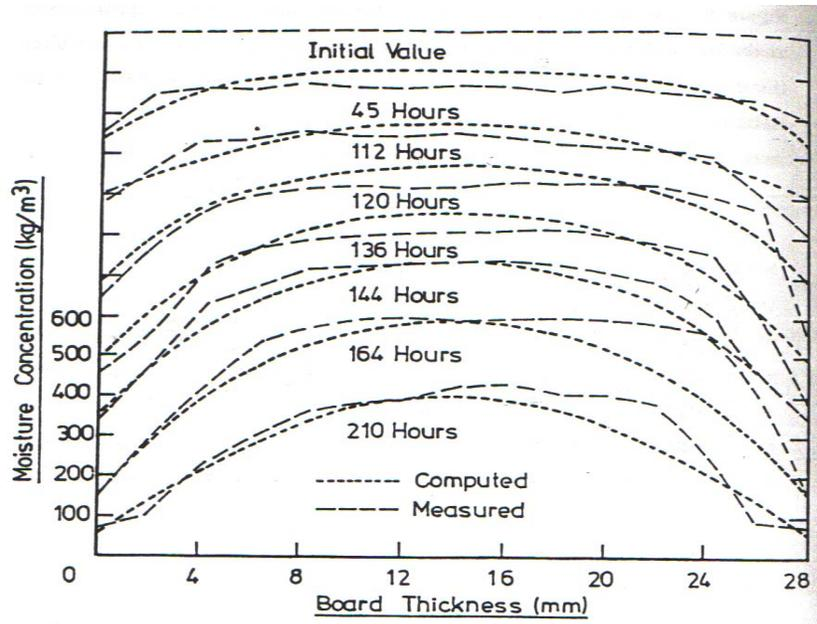
**Figure 2.5.** Parabolic moisture profiles, throughout the drying process of Tasmanian eucalypt timber, predicted by the diffusion model and measured experimentally (Wu, 1989).
