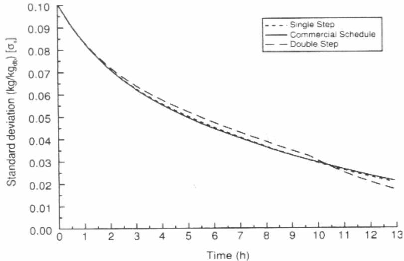
**Figure 2.2.** Standard deviation of moisture content as a function of time for a single set point schedule, double set point schedule, and a commercial schedule (Cronin *et al.*, 2003).
