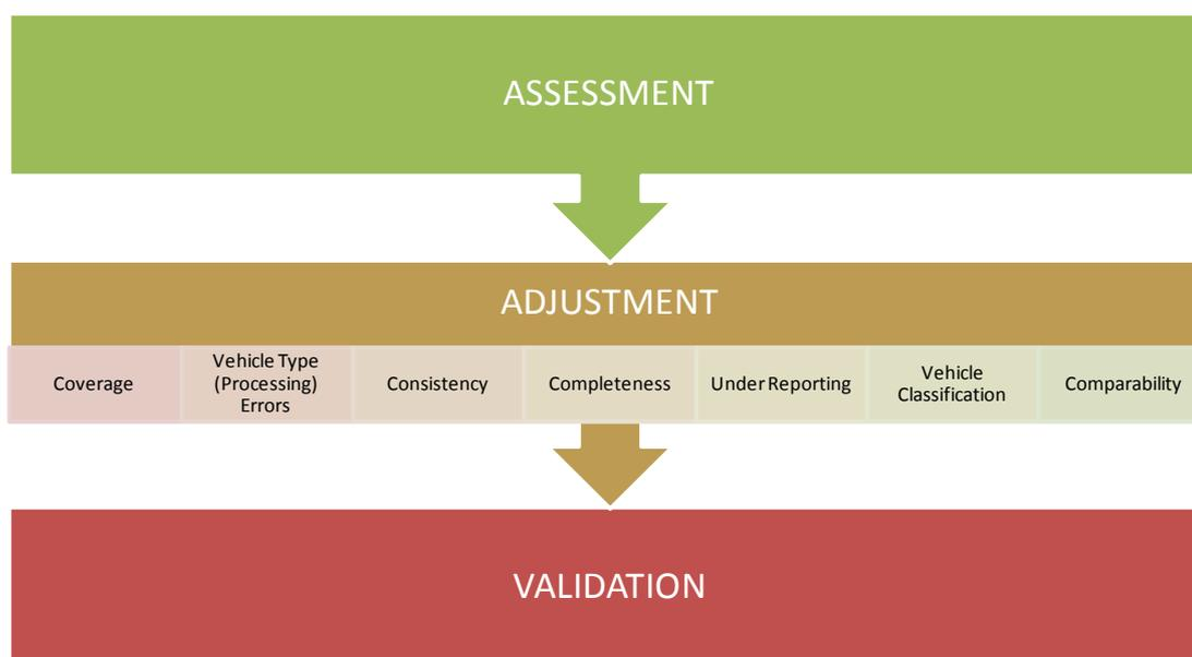
Figure 2: Motor vehicle data correction framework
